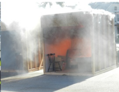
Both structures had smoke detectors and burned freely. On the left, the structure with sprinkler was saved on the right without was heavily damaged. and SPARKY was ther too!
