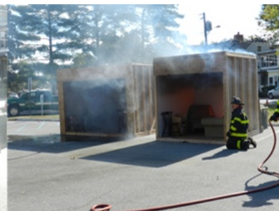
Both structures had smoke detectors and burned freely. On the left, the structure with sprinkler was saved on the right without was heavily damaged. and SPARKY was ther too!
